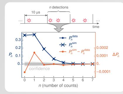
A sample measurement of the probability distribution of the number of counts in a 10-µs window.
