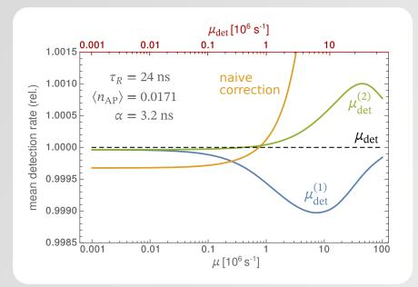
Assessment of mean rate accuracy as a function of incident rate [1]. The baseline is the point process model. Parameters (from top) are recovery time, mean afterpulses per detection, and the twilight coefficient.
