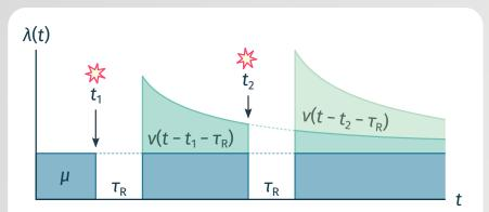
SPAD counting as a self-exciting point process. The intensity  $\lambda$  in time consists of a constant intensity  $\mu$ and afterpulsing contributions v triggered by the detections. (scale exaggerated)
