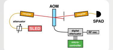
Acousto-optical intensity modulation: 32 dB dynamic range, 128 levels, 300-ns response Accuracy ~  $10^{-4}$ Works identically for pulsed light Det. recovery time « det. window « modul. period « meas. time 23 ns 10 µs 1 ms 100 s
